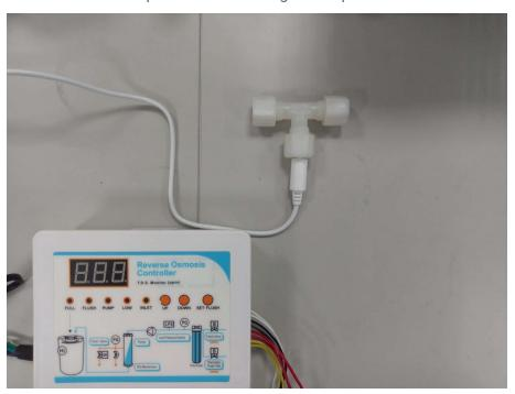
5. Connect the Black wire to the flush solenoid valve or motorized valve (110V/220V)
